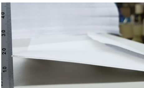
Curled or Twisted - Drive the bottom corner (double spacers or remove s pacer from leading corner)
